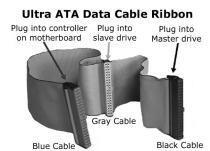
Please note the configuration of the internal ATA cable already installed in your existing system. If your internal cable is configured differently than pictured here, you may want to replace it before installing a new hard drive to achieve maximum performance.
